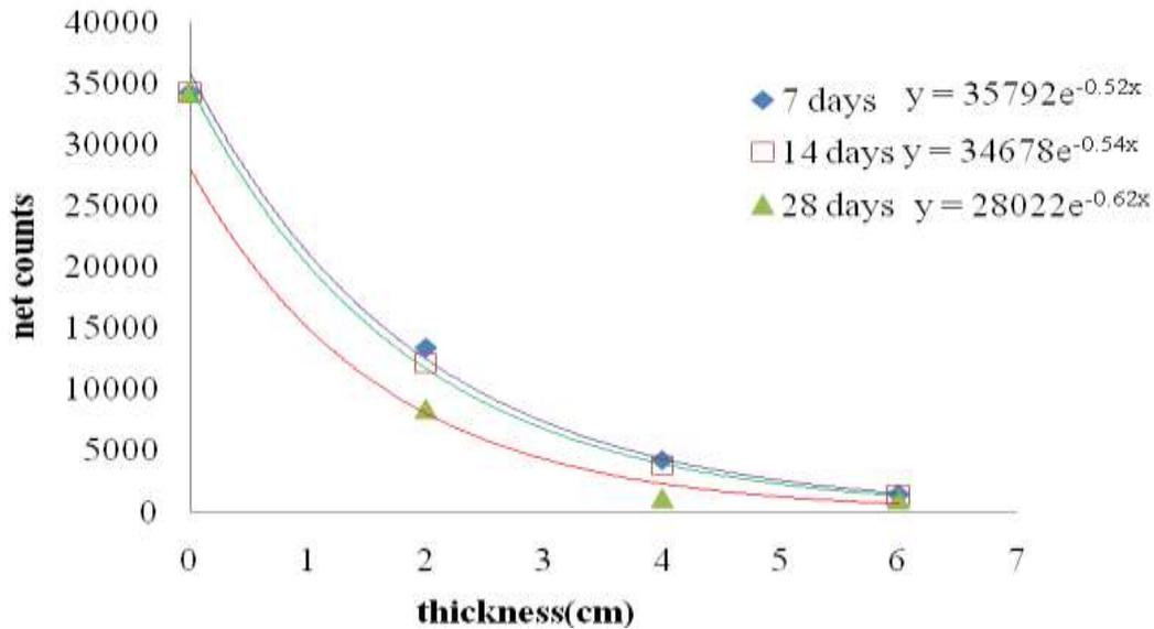
**Figure (8) The variation of gamma counts with the thickness of 30 MPa concrete sample**
