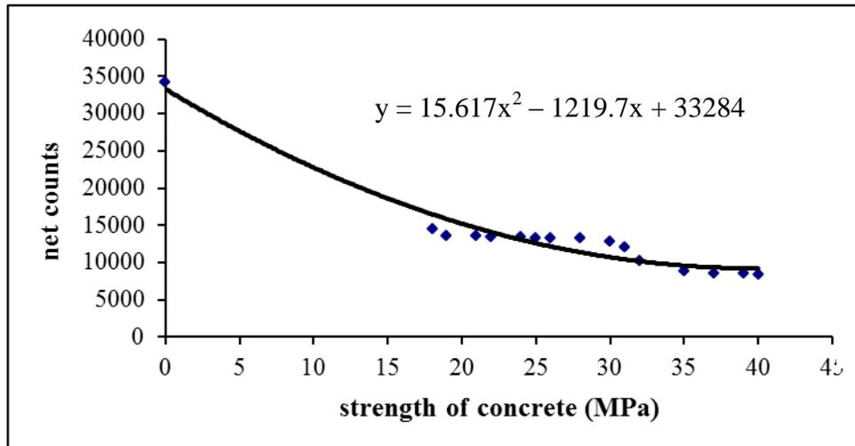
**Figure (3) The variation of gamma counts with the actual strength of concrete samples**
