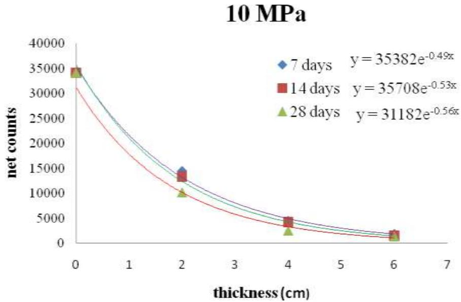
Figure (4) The variation of gamma counts with the thickness of 10 MPa concrete sample
