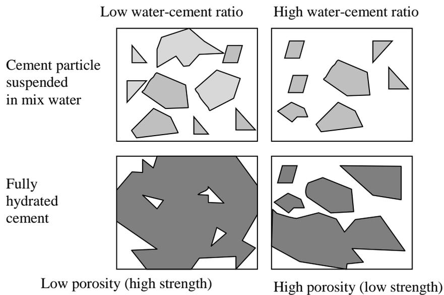
**Figure (2) Schematic drawings to demonstrate the relationship between the water/cement ratio and porosity**
