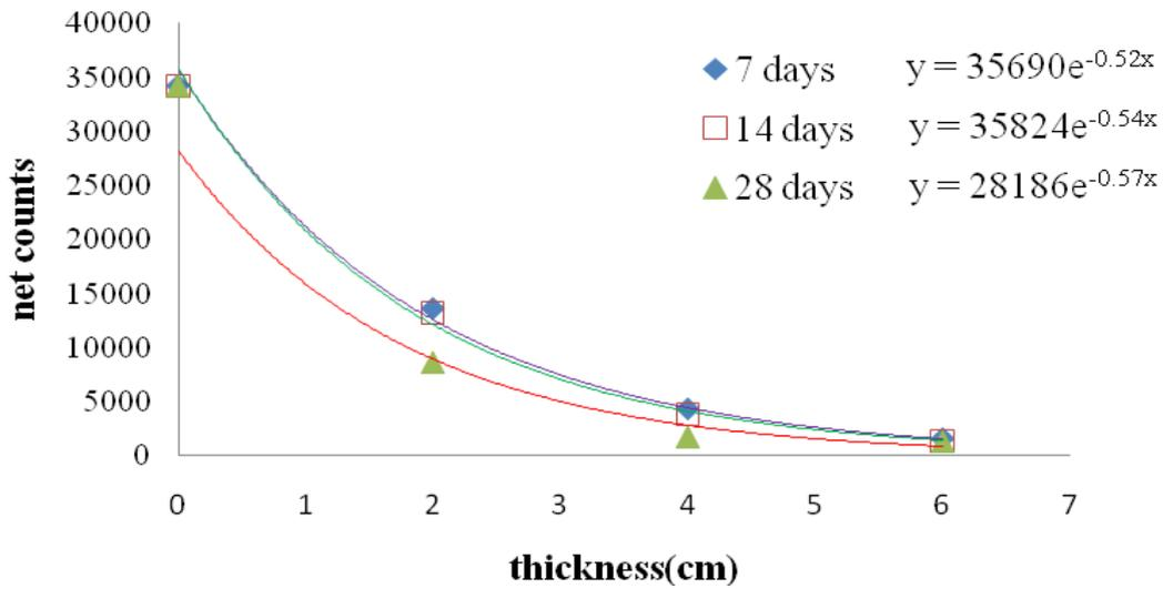
Figure (6) The variation of gamma counts with the thickness of 20 MPa concrete sample
