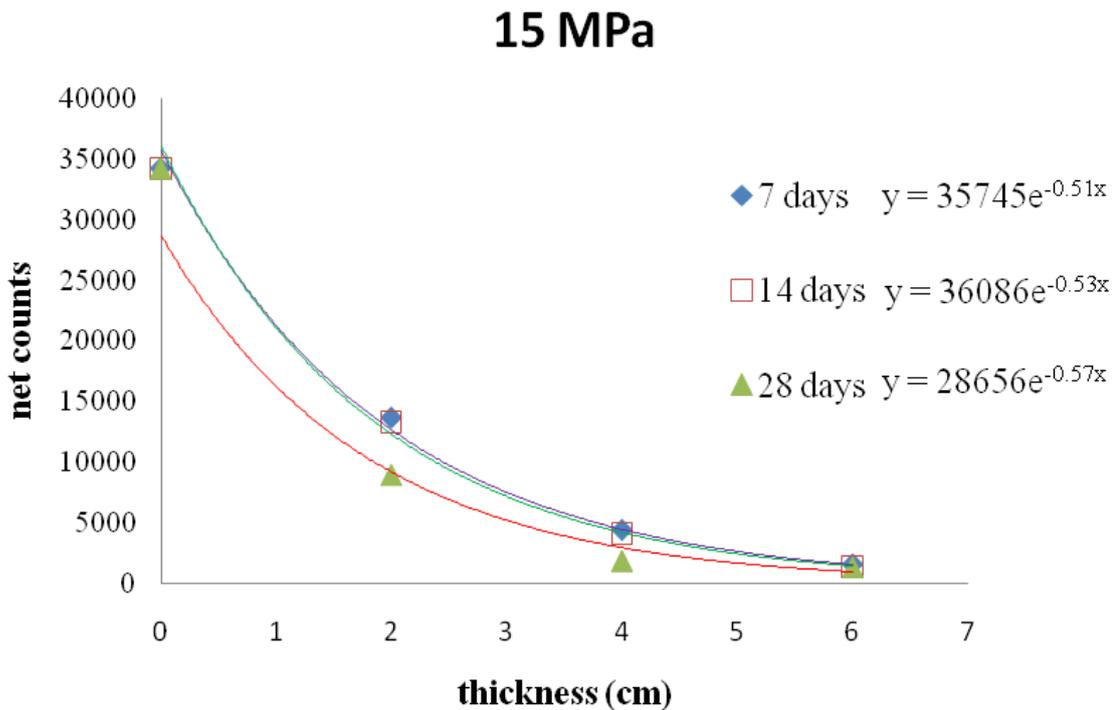
Figure (5) The variation of gamma counts with the thickness of 15 MPa concrete sample
