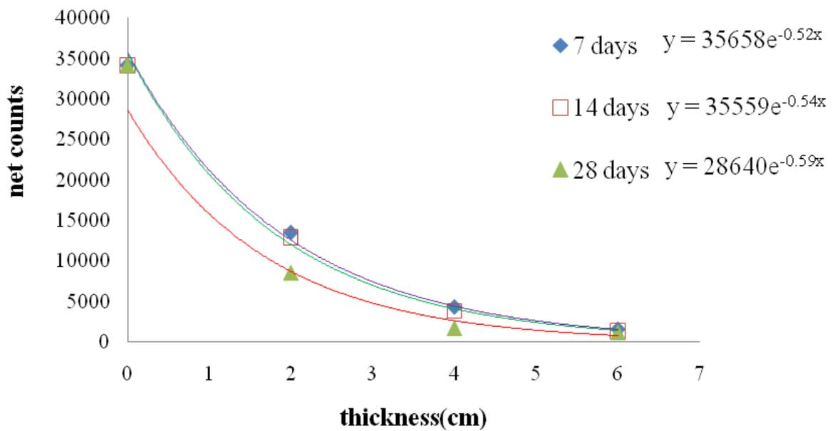
Figure (7) The variation of gamma counts with the thickness of 25 MPa concrete sample
